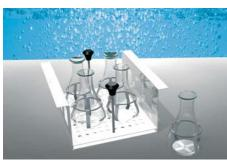
Retaining elements for conical flasks and test tubes (for shaking device)
