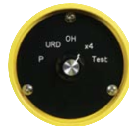
Switch face found for the VDA040P probe.
